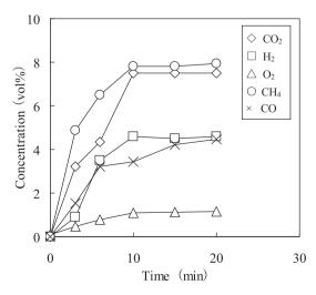
Fig. 5 – Changes of gas concentrations during acetic acid decomposition over the porous dolomite pellets (bed temperature: 800  $^\circ$ C, gas residence time: 7.5 s). Y. Miao et al.
