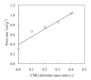
Fig. 3 – Changes of pore rate with CMC/dolomite mass ratio of the porous dolomite pellets (clay/dolomite mass ratio: 0.4). Y. Miao et al.
