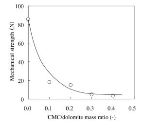
Fig. 2 – Changes of mechanical strength with CMC/ dolomite mass ratio of the porous dolomite pellets (clay/ dolomite mass ratio: 0.4). Y. Miao et al.
