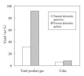
Fig. 8 – Comparison of the yields of total product gas and coke in acetic acid decomposition over different catalysts (bed temperature: 800 °C, gas residence time: 7.5 s). Y. Miao et al.
