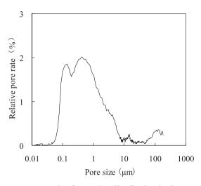
Fig. 4 – An example of pore size distribution in the porous dolomite pellets (CMC/dolomite mass ratio: 0.2, clay/ dolomite mass ratio: 0.4). Y. Miao et al.
