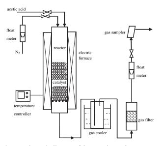
Fig. 1 – Schematic diagram of the experimental apparatus. Y. Miao et al.
