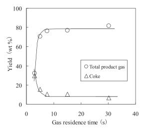
Fig. 6 – Effect of gas residence time on acetic acid decomposition over the porous dolomite pellets (bed temperature: 700  $^{\circ}$ C). Y. Miao et al.
