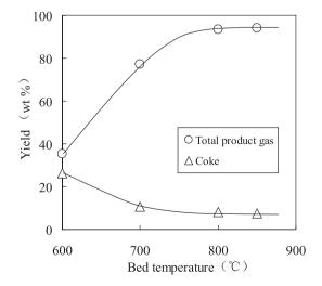
Fig. 7 – Effect of bed temperature on acetic acid decomposition over the porous dolomite pellets (gas residence time: 7.5 s). Y. Miao et al.
